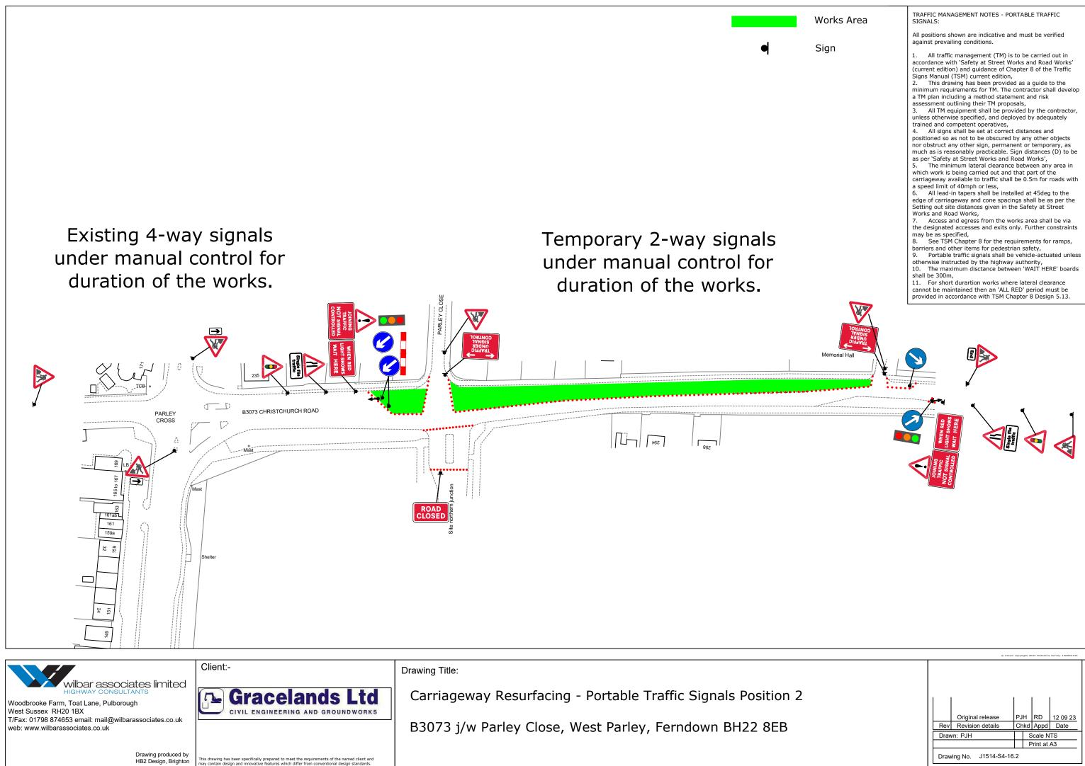
drawing has been specifically prepared to meet the requirements of the named client and contain design and innovative features which differ from conventional design standards.
